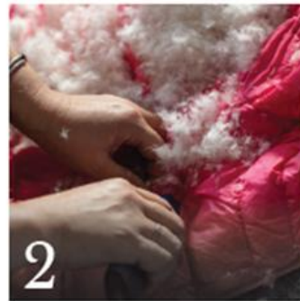
2 Extracting Mechanical extraction of the down and feather from the shell.
